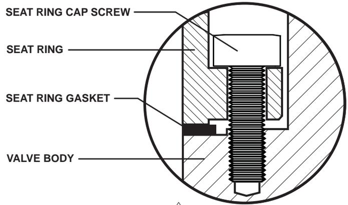
**Figure 5** Detail B - Seat Ring Gasket
