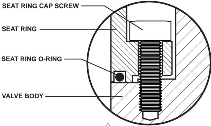
**Figure 4** Detail B - Seat Ring O-Ring
