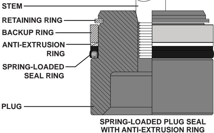
**Figure 6** Detail A - Model 380 Plug Seal Options
